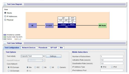
Landslide supports numerous VoLTE IMS interfaces (Cx, Gm, I2, ISC, MI, Mw, Mx, Rx, Sh, SIP-I/T, Ua/Ub, Ut ...). Furthermore, the Landslide Generic IMS Trunk Interface emulation allows the user to emulate any SIP interface between IMS sub-components by creating a new SIP call flow using existing Landslide SIP Supplementary actions and adding new headers and/or fields to the SIP messages as required.
