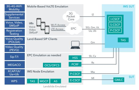
The Landslide LTE Gateway Test Application combined with the VoLTE/IMS feature provides a means of testing LTE gateway performance using data traffic, VoLTE calls or both. Integrated support for the Rx interface from the IMS node or SIP Proxy provides a means of testing PGW and/or PCRF operation and performance when using dynamic policy and charging control for dedicated bearer creation, modification and deletion.
