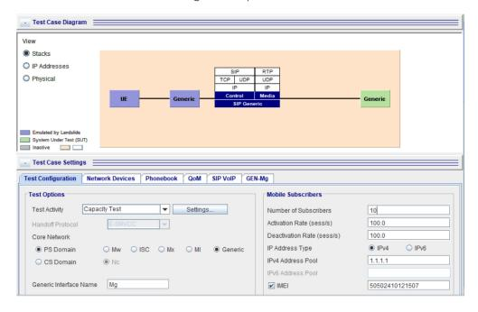
Landslide's MCPTT testing capabilities and feature set enable testing of Private Calls (on network), Group Calls (on network), MCPTT Client authentication using OIDC (OpenID Connect), MCPTT Configuration Management and MCPTT Floor control as defined by 3GPP MCS framework. Supported interfaces include: CSC-1, CSC-4, MCPTT-4, MCPTT-7 and Rx for MCPTT.
