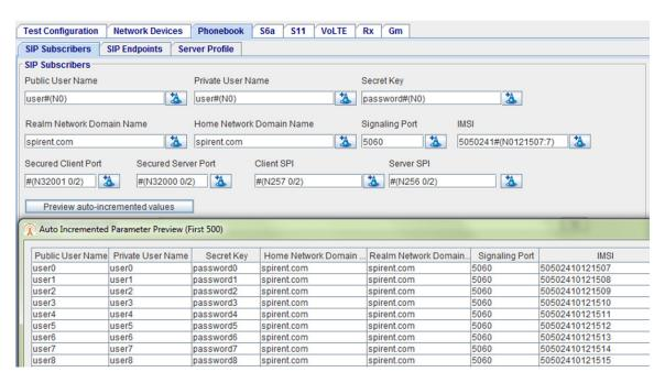
The IMS Node emulation provides a standalone SIP proxy/P-CSCF emulator that can emulate SIP end points or the proxy function and drive the Rx interface to the PCRF.
